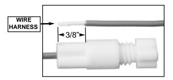
NOTE: If the strip length is too short, the connector will not function properly. The stripped portion of the wire must extend beyond the locking mechanism.
