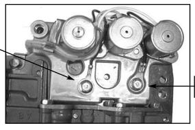
Shift Solenoid ground wires
