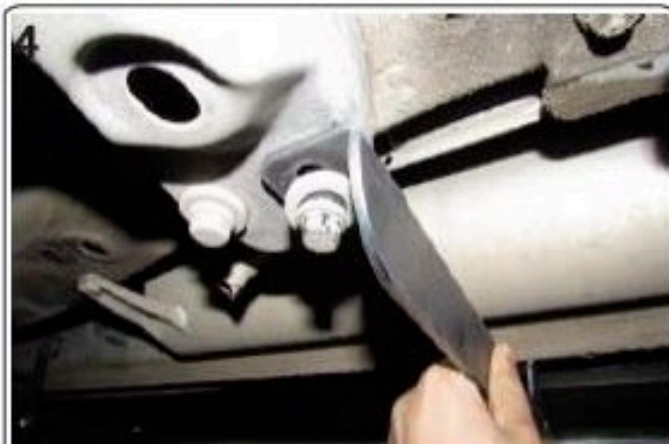
4) Install using factory bolt
