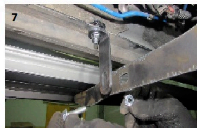
7) Attach brackets together hand tight
