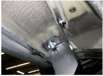
1) Locate front mounting area and install front bracket as shown above. Do not tighten yet.
