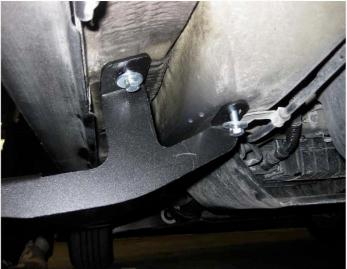
Locate middle bracket mounting area and install middle bracket as shown above. Do not tighten yet.
