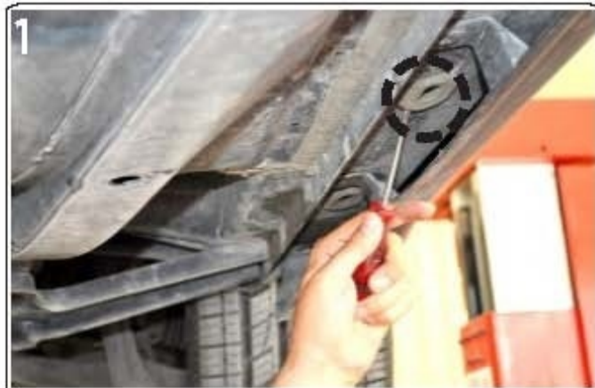
1) Locate front mounting position, note this is the second hole from front to back
