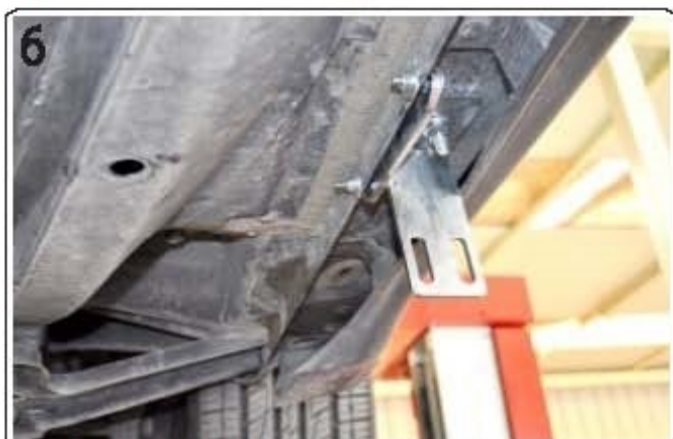
6) Bracket properly installed
