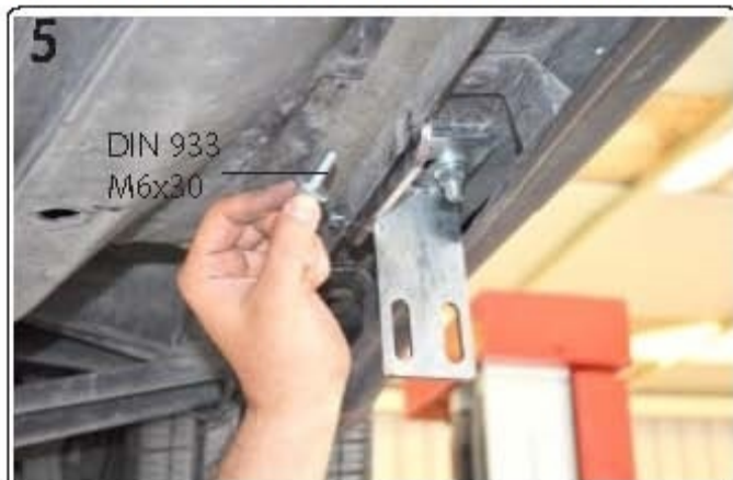
5) Attach bracket with M6 bolts to not tighten
