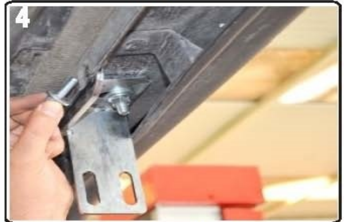
4) Attach bracket with supplied M6 hardware
