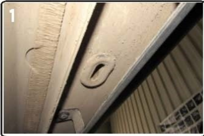
1) Locate middle bracket mounting point 3rd hole
