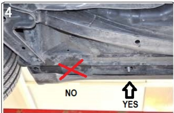
4) Notice correct insert position
