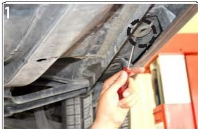
1) Locate front mounting position, note this is the second hole from front to back
