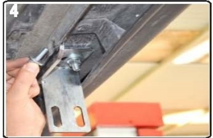
4) Attach bracket with supplied M6 hardware
