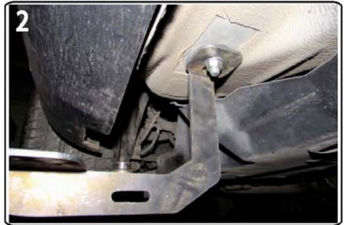
2) Attach rear mounting bracket as shown above
