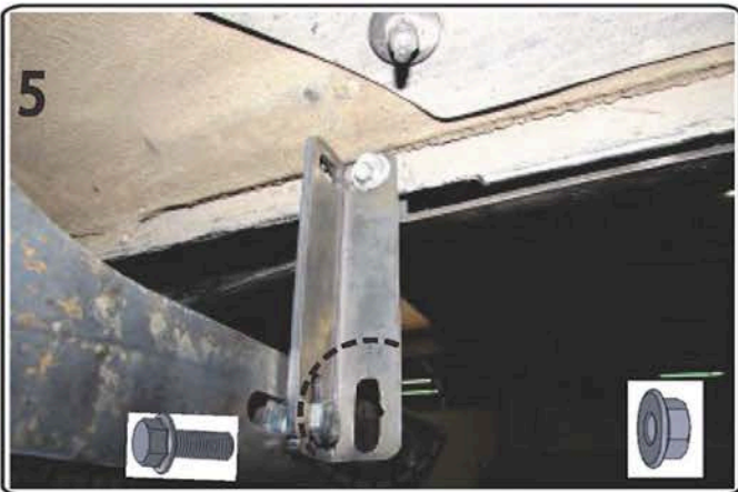
5) Install hardware on upper extra support mounting point do not tighten, you are now ready for the rear bracket.
