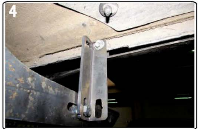
4) Attach extra support bracket with supplied hardware M6
