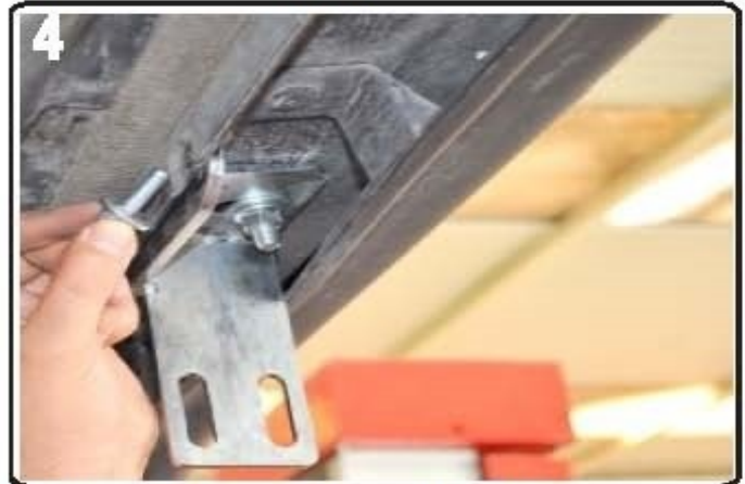
4) Attach bracket with supplied M6 hardware
