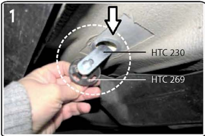
1) Locate rear bracket mounting point insert HTC 230 with HTC 269
