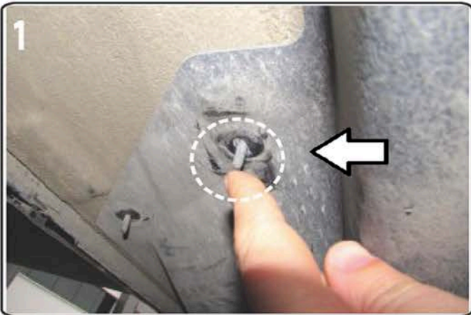
1) Locate front bracket mounting point, if equipped remove factory nut
