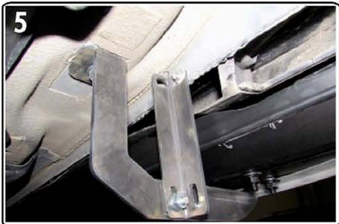
5) Loosen M8 hardware on back of steps
