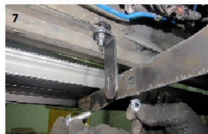
7) Attach brackets together hand tight
