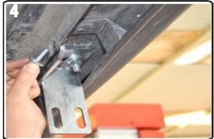
4) Attach bracket with supplied M6 hardware
