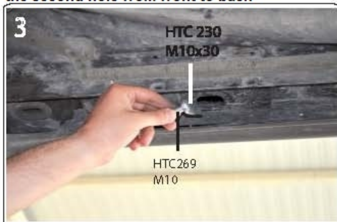
3) Insert HTC 230 with HTC 269 as shown
