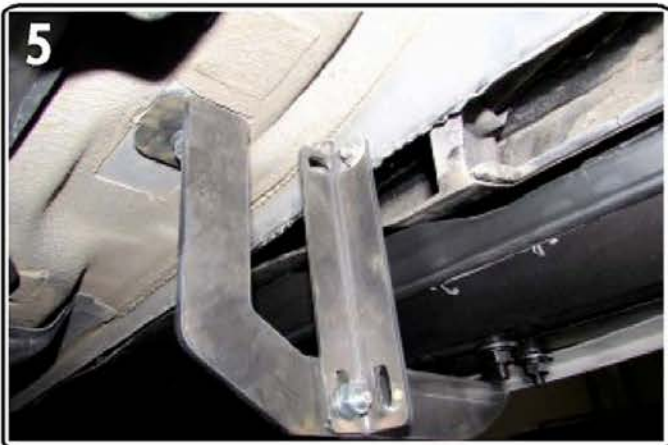
5) Loosen M8 hardware on back of steps 6) Attach steps to brackets hand tight only 7) Proceed to tighten brackets M6 to 8 ft lbs M8 to 18 ft lbs and M10 to 35 ft lbs 8) Proceed to tighten setps hardware M8 to 18 ft lbs
