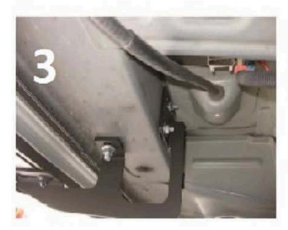
3) Proceed to install front bracket as shown on PIC #3 bracket hardware must be hand tight only
