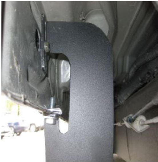
1) Insert M8 Nut on vehicle pinch weld
