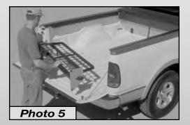
outboard to permit the wheels to enter the Tracks (*Photo 4*). Next, maneuver the Cargo Manager Divider around the back bed posts and rotate the Divider to insert the lead wheel on each side (*Photo 5*). With the lead wheels in place, squeeze the Linkage Control Levers to retract the linkage and rotate the Divider to the vertical position, then align and insert rear wheels. With the wheels in place, press the Track Stop Pins inboard to prevent the wheels from leaving the Tracks.
