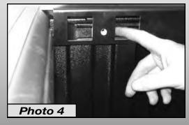
between the knockouts so the holes line up *(Photo 4)*. Use 1/4 - 20 x 1" counter-sunk screws to secure the Adapter Flange to the bulkhead.
