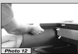
fin on the underside of each Track seats into the slot in the Clamps (Diagram 13).
