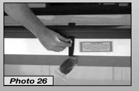
■ To open the Cover pull back slightly on the Handle to relieve spring tension from the Latch Mechanisms and turn the Lock Lever clockwise to the 10 o'clock (unlatched) position.
