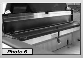
of space between the bulkhead and the back of the Housing. **Do not fasten** the Housing in place.
