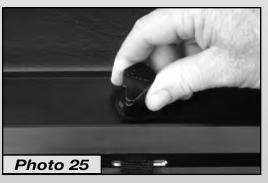
wing nut and detach the Pull Strap from the threaded stud *(Photo 26)*. Pull the Cover closed and latch it to the tailgate. **Note: Do not allow the Cover to retract while the Housing Lid is open.**
