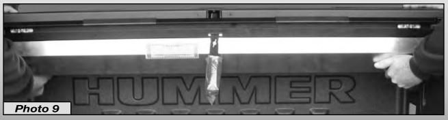
A. Place the Housing Assembly onto the Housing Brackets and Bulkhead Flange (*Photo 9*).
