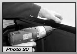
This should be a snug fit. While holding the Tailgate Extrusion in place, use a #8 x 3/4" self tapping screw and power screw gun to secure the center hole *(Photo 20)*.
