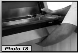
slightly on the Housing and shift each side back toward the tailgate *(Photo 18)* so that the Track End Caps contact the inside surface of the tailgate. Make sure the Track End Cap metal blocks contact the Tailgate Extrusion End Cap.
