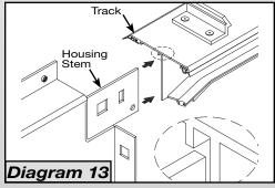
(Photo 12) and key them onto the Housing Stems (Diagram 13), being sure that the Handle is properly engaged into the Tracks.
