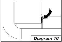
the inside surface of the tailgate. Make sure the Track End Cap Metal Blocks contact the Tailgate Extrusion End Caps (*Diagram 16*). Note that if the Tracks are not positioned as shown, the Latch Mechanism will not function correctly.
