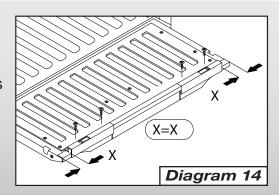
**C.** With the Tailgate Extrusion secured, carefully close the tailgate, being cautious not to strike the ends of the Tracks.
