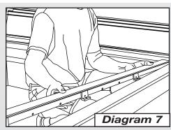
B. Unwrap the Tracks and locate the supplied Bed Clamps that are taped together along with the bolts and washers. Unwrap the Clamps and set them in the bed of the truck. Carefully place the Tracks on the bedrails (*Diagram 7*) and key them onto the Housing Stems (*Diagram 8*), being sure that the Handle is properly engaged into the Tracks.
