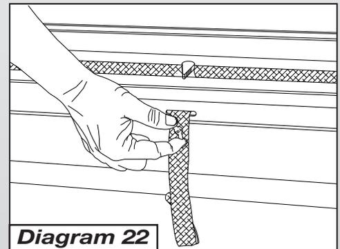
D. To open the Cover pull back slightly on the Handle to relieve spring tension from the Latch Mechanisms and turn the Lock Lever clockwise to the 10 o'clock (*unlatched*) position, while holding the pull strap allow the Cover to retract back into the housing with just enough force to reset the Lock Lever.
