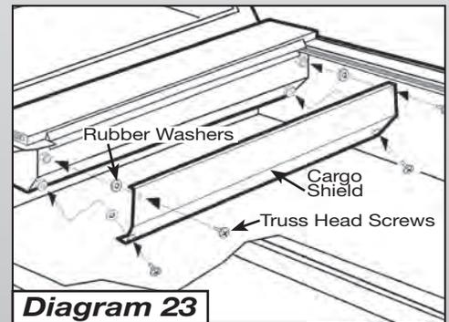
E. Use the 14-20 x 1/2" truss head screws and rubber washers supplied to secure the Cargo Shield (**Diagram 23**).
