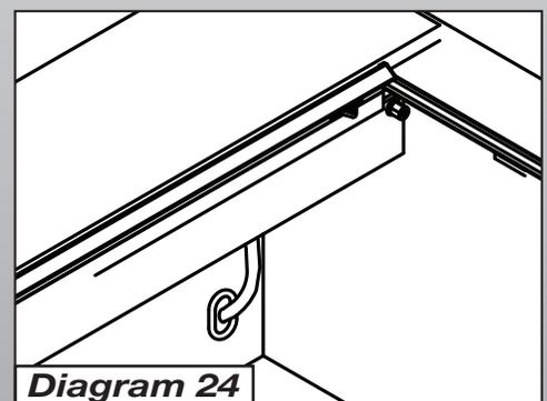
G. Always make sure the Pull-Strap is securely clipped to a fixed point in the bed.
