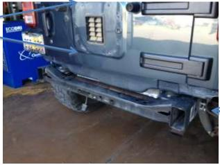
Arrows indicate frame side bolts (2 per side) and tire carrier (4 per side)
