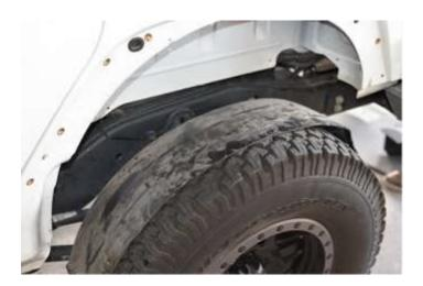
11. Tuck wheel well liner behind the fender flare and under lip. Attach liner to stock locations using stock push-in plugs or provided push-in plug at the factory attachment points
