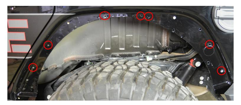
Install the rear brackets as shown: D5 will be installed towards the front on the lower portion of the fender well using **two** 1/4" - 20 flanged bolts..
