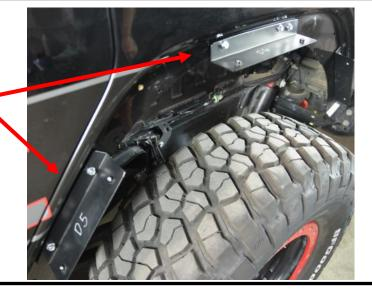
D7 will be installed at the rear of the fender well on the lower portion using **two** 1/4" - 20 flanged bolts.
