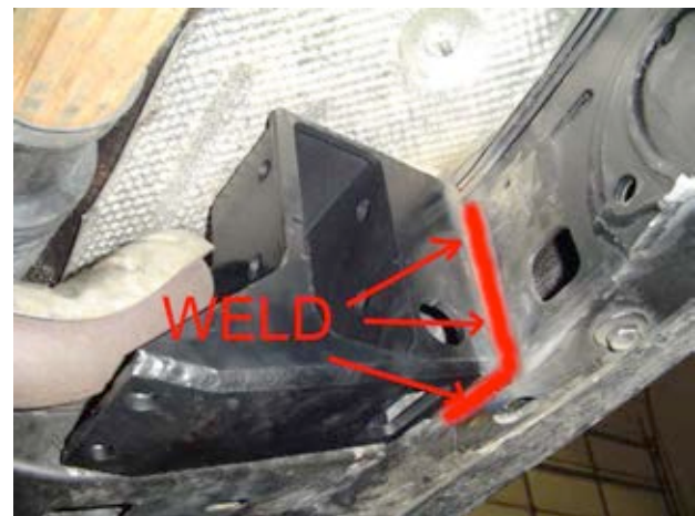
D.S. Bracket Welded in Place
