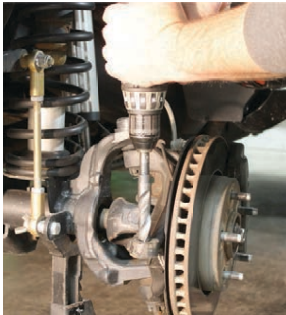
Drilling out knuckle to 18mm
