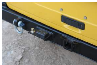
2" TOW RATED RECEIVER + SAFETY CHAIN HOOKS
