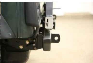
3/16" THICK STEEL TUBE 2" X 4" CONSTRUCTION
