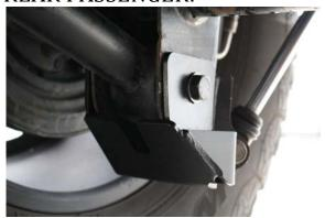
3. Install skid plate over control arm mount and align holes.
