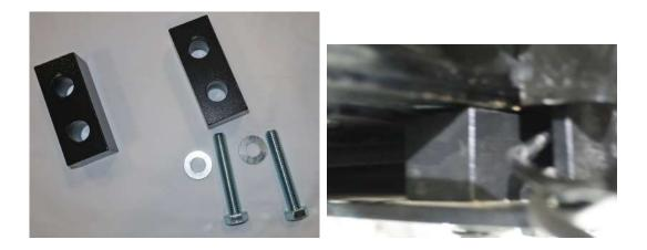
5. Install 2x 14MM x 1.50 x 40MM bolts with flat washer from outside of frame onto each side. 22MM socket with short extension. Tighten all hardware.
