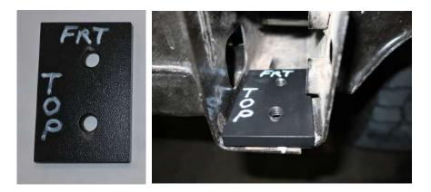
4. Set top lip of bumper on frame. Slide 2x 1-1/2" x 5/8" x 3-1/4" blocks with 2 holes between frame and lower lip of bumper. Make sure wiring is between bumper and block and will not get pinched. Use 2 factory bolts from tow hook on driver side. Use 2-1/2" x 3" full thread bolts with 2x 1/2" SAE flat washers on passenger side 18MM wrench on factory bolt using ¾" wrench on ½" x 3" bolts. Do not tighten fully.
