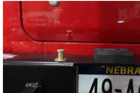
(Striker nut installed)
