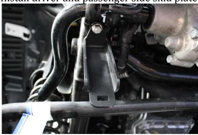
PRO TIP: Some skid plates actually install easier if you install front of skid first. Skid to step 8.
