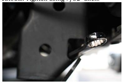
8. Install remaining 2x 3/8" bolts with washers from bottom side up (threads inside bumper cavity) and secure using 3/8" nylock nuts and 9/16" wrench.
