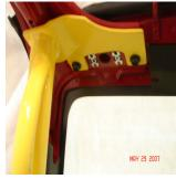
10. Use drill guide to mark where to drill holes. Top of drill guide should be lined up with top of nut plate that is welded to dash side plate. Center punch holes or mark with sharpie. Remove a-pillar upright (unbolt from top of windshield as well) and drill holes using long drill
