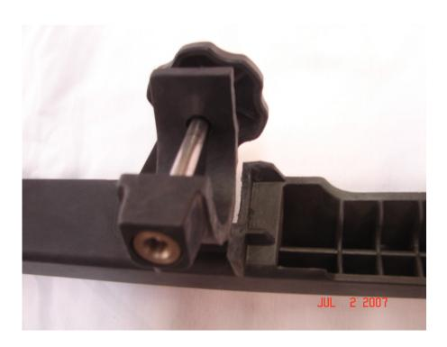
HARD TOP: Some hard tops need to be trimmed as front overhead corner clamps rub fiberglass top. This causes an improper seal and creates wind noise. The thickness of the fiberglass varies up to 1/4" due to variations in fiberglass cooling times and manufacturing facilities. To trim fiberglass –
