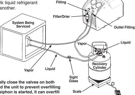
WARNING: Manually close the valves on both the storage cylinder and the unit to prevent overfilling the cylinder. Once the siphon is started, it can overfill the storage cylinder, even if the cylinder is equipped with a float level sensor. The siphon can continue even when the unit is turned off.
