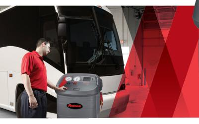
The Robinair 17800C recovers, recycles, evacuates and recharges, multiple refrigerants all in one fast and continuous operation through one hook-up. It's ideal for mass transit vehicles, buses, refrigerated trailers or containers and other applications that use a refrigerant other than R134a and not typically found in mobile applications.
