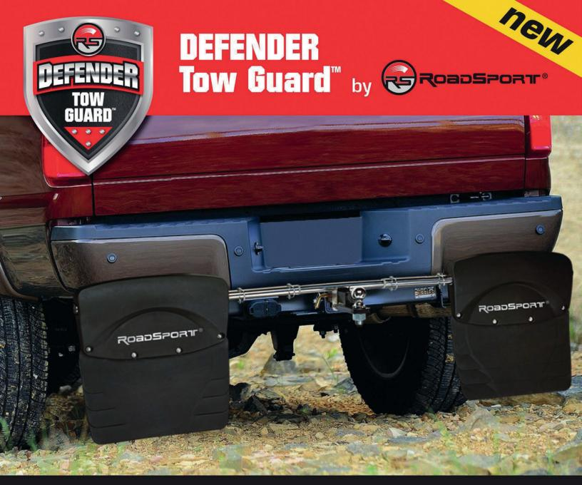
Protect your investment with the ultimate towing protection guard on the market today. Fully adjustable to fit all trucks, including dually pick-up trucks, with 2" trailer receivers. Mounts directly to the trailer draw bar. Mud guards offer a quick connect and quick release system. 24" tall mud guards can be trimmed to desired height. Made from heat resistant materials. Stainless Steel bar construction.
