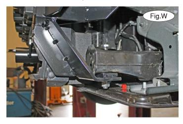
15. On each side, place a  $\frac{1}{2}$ " plate washer over a  $\frac{1}{2}$ " x 4" bolt and bolt down through the subframe and main receiver brace. Finish with a  $\frac{1}{2}$ " lock washer and nut (Fig.W). *Note:* due to manufacturing variances, some applications may require bolting up through the main receiver brace and subframe instead.
