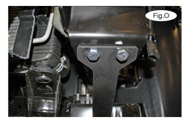
12. Using two of the supplied ½" x 1¼" bolts, lock washers and nuts, bolt the lower rear brace to the main receiver brace (Fig.O). Tighten the bolts to the bolt torque requirements found at the end of this document. *Note:* use Loctite® Red on all nuts and bolts.
