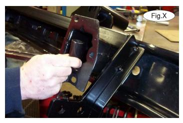
20. Place a 1" x 2" pipe spacer inside the bumper core (Fig.X). Bolt through the main receiver brace, bumper core support and the pipe spacer using a  $\frac{1}{2}$ " x 5" bolt.
