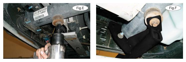
3. Remove the 19mm frame mounting bolts (Fig.E). There is one on each side.
