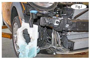
6. On the passenger side only, pull up and out to release the filler neck. Remove two T30 Torx (head) bolts attaching the top of the washer bottle to the frame (Fig.H). Then, carefully lift the washer bottle out and maneuver the washer bottle around the framing. Secure the bottle away from the frame for now (Fig.I).
