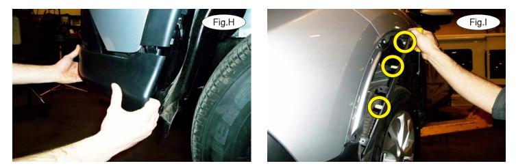
5. On each side, carefully pull the lower fascia from the fender trim (Fig.H), and the fender trim from the fender (Fig.I), releasing three clips.
