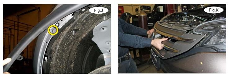
7. With a firm grip on the grille, pull hard and straight out on it to release it from the two yellow clips near the headlights and the four yellow clips along the bottom of the grille (Fig.K). On each side, pull out on corner of the fascia to remove it from the locking strip as indicated by the yellow lines in Figure L) and then a screwdriver to release the yellow clip shown in Figure M.
