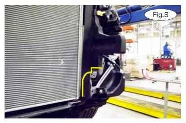
13. Trim the passenger side air dam as shown in Figure R and the driver's side air dam as shown in Figure S.
