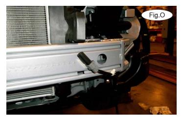
8. Now, pull out and forward to remove the fascia. Disconnect the fog lights, if the vehicle is so equipped.
