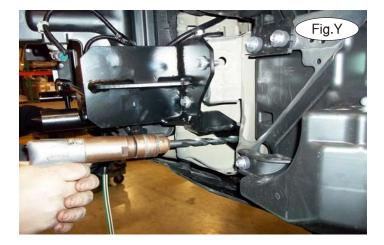
18. Working on the driver's side only, using the lower mounting point of the main receiver brace as a template, drill a ½" hole through the two layers of the frame rail (Fig.Y). *Note:* use caution to avoid drilling into the cooling line.
