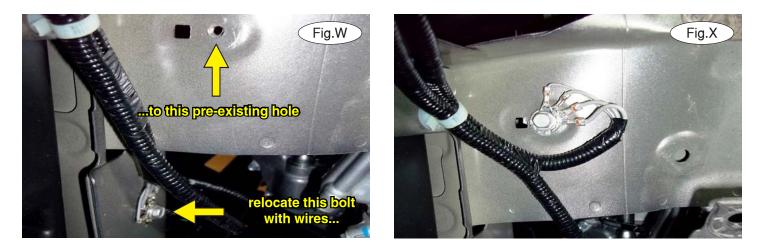
16. Now, pull back the fender liner and remove the 10mm (head) bolt with wires (Fig.W). Relocate it to the pre-existing threaded hole about six inches up on the side of the frame (Fig.X).
