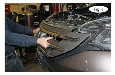
7. With a firm grip on the grille, pull hard and straight out on it to release it from the two yellow clips near the headlights and the four yellow clips along the bottom of the grille (Fig.K). On each side, pull out on corner of the fascia to remove it from the locking strip as indicated by the yellow lines in Figure L) and then a screwdriver to release the yellow clip shown in Figure M.
