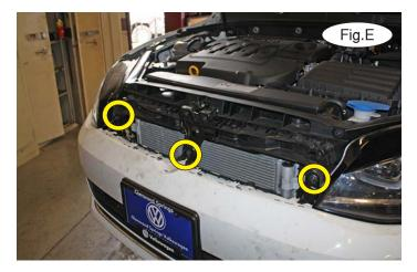
2. Remove three T30 Torx bolts attaching the upper fascia to the core support (Fig.E).
