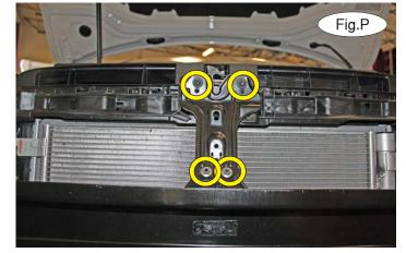
10. Remove two 10mm nuts and two T30 Torx bolts attaching the core support bracket to the bumper core (Fig.P). Set it aside for now.
