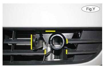
19. Trim the fascia as shown in Figure Y to allow clearance for the main receiver brace.
