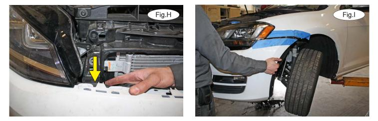
5. Reach in behind the fascia and disconnect the fog lights, if the vehicle is so equipped. Then, on each side, locate the plastic tab indicated by the yellow arrow (Fig.H – passenger side). Pull out on the corners of the fasciato release the locking strips while releasing the tabs (Fig.I).
