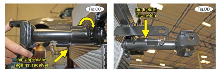
22. On each side, insert the removable front bracket arm into the front receiver 90 degrees from its final towing position, depressing the spring-loaded pin against the receiver (Fig.BB). Now, twist back 90 degrees until the spring-loaded pin snaps into place in the notch on the receiver, locking the arm into place in its final towing position (Fig.CC).
