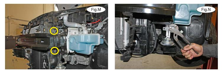
7. Support the core support with a jack stand. On each side, remove two T30 Torx bolts attaching the core support to the bumper (Fig.M).
