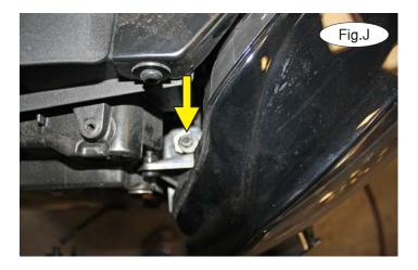
6. On each side, there are four T30 screws attaching each headlight to the frame. Remove three and loosen one (Fig.J, K and L – driver's side). Disconnect each headlight and set it aside for now.
