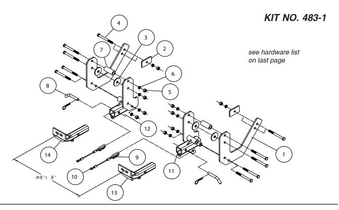
**IMPORTANT:** All brackets **must** be assembled with all the bolts left loose for final adjustment and positioning (before tightening) unless otherwise instructed. All bolts **must** be torqued for proper strength. If more than one bolt is used per fastening point, the diagram may only show one.
