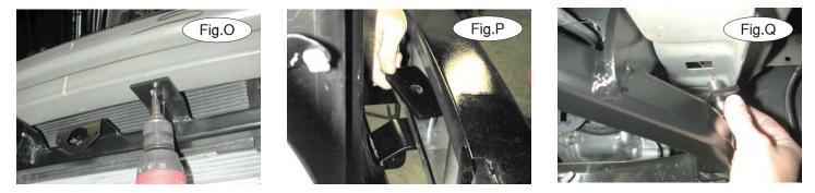
11. Using the pre-drilled holes in the main receiver brace as a template, drill two 1/2" holes through the bumper core (Fig.O).
