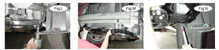
9. Lift the main receiver brace into place, and attach it to the subframe with the factory subframe bolts you removed in step 8, using thread lock (Fig.N). Torque the bolts to the specifications listed at the end of these instructions.
