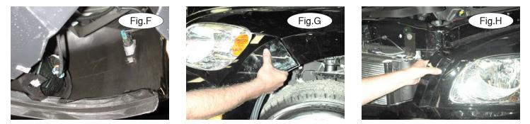
4. Pull back the fender liner to gain access to the fog lights and side marker lights. Unplug them and repeat for the other side (Fig.F).
