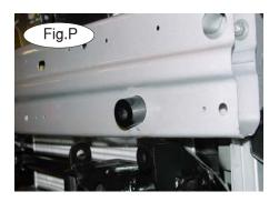
11. Insert two 1/8" pipe spacers in the large bumper core holes and bolt through the spacers, upper brace plates and frame with  $\frac{1}{2}$ " x 4" bolts, flat washers, lock washers and nuts (Fig.P,Q,R).
