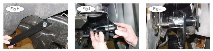
7. Bolt through the receiver brace and frame and finish with  $\frac{1}{2}$ " nuts and lock washers (Fig.J).
