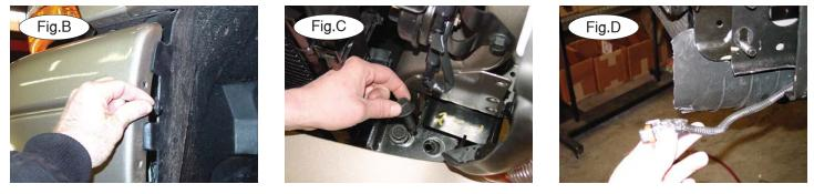
Remove three torx screws in each fender well (Fig. B). Disconnect the fog lights, if the vehicle is so equipped (Fig.D). Then, remove four bolts, two on the top of each frame tube (Fig.C). Now, remove two bolts on the bumper side braces on each side. These are located on the sides of the frame tubes.
