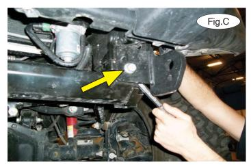
4. Fit the main receiver brace around the lower subframe, aligning the lower holes with the pre-existing holes in the subframe. Use a support stand, if necessary.
