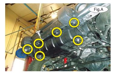
1. Remove four 13mm (head) bolts and two 15mm (head) nuts and bolts attaching the skid plate to the bumper (Fig.A). The skid plate will not be replaced. Retain the skid plate and attachment hardware for replacement in case the bracket is ever removed.
