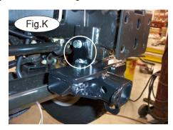
5. Place a ½" lock washer over a ½" x 1¼" bolt. Place a 3/16" x 1½" x 3½" threaded backing plate with wire through the opening on the inside edge of the frame rail (Fig.J) and bolt through the main receiver brace, frame rail and into the backing plate (Fig.K).
