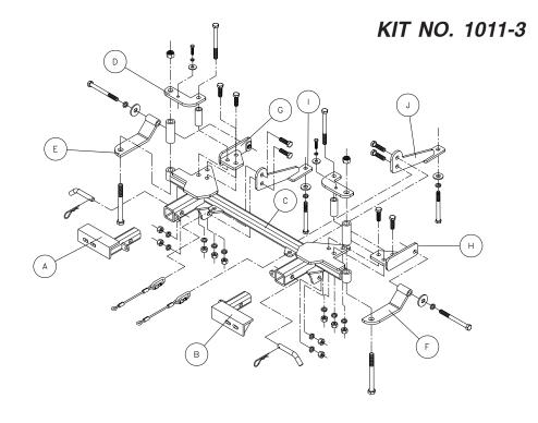
**IMPORTANT:** All brackets **must** be assembled with all the bolts left loose for final adjustment and positioning (before tightening) unless otherwise instructed. All bolts *must* be torqued for proper strength. If more than one bolt is used per fastening point, the diagram may only show one.
