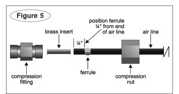
Next, slide one of the brass inserts (Figure 5) into the end of the line.
